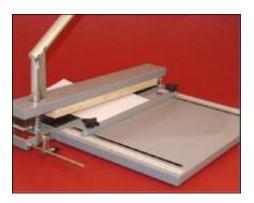
You can mount the MA-500 table to the IBK-32 multifunction press with two M6 screws.
