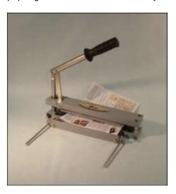
This simple paper guide has no scale it is a bit complicate to set the proper position. You can crease much more comfortable and accurate using the MA-500 work table for this press.
