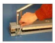
Mount the side paper guide (4) to the machine use an M6 washer and fix it. You can mount the side paper guide to any side of the machine.
