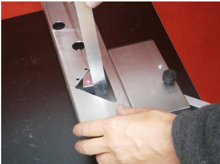
Insert the edge protector guide into the device as in the picture.
