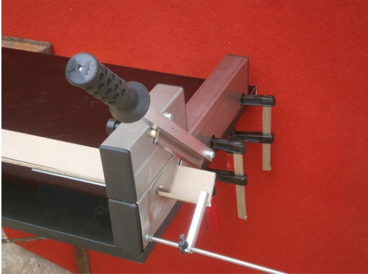
If you positioned the edge protector to the desired position, release the safety pin with pulling its knob.
