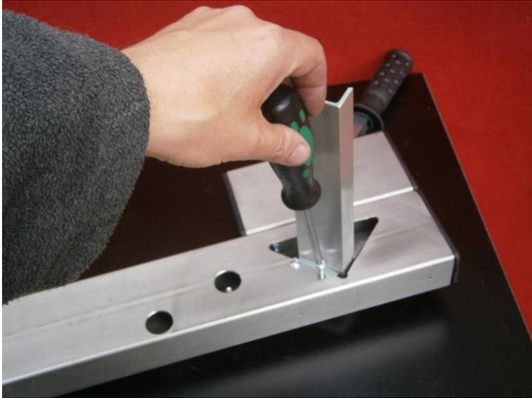
Fix it with two M4 screw. Adjust the guide before fixing the screws so that you can push the edge protector through the EVV-2 without hit the frame of the device.
