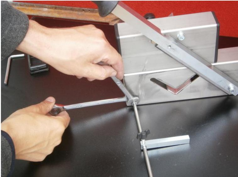
And mount the paper stop as in the picture. Press back the end plug and fix the EVV-2 edge protector cutter to a table with the two clamps which are delivered with the device.
